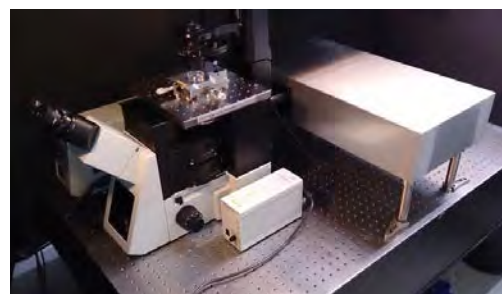
A prototype of a super resolution microscope (SAX microscope).
