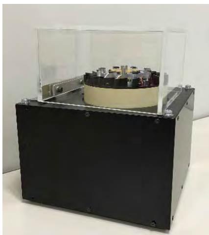
Microchip (top) and device (bottom) prototype. This chip can take in the needed volume of sample and can do rapid PCR on the device.
