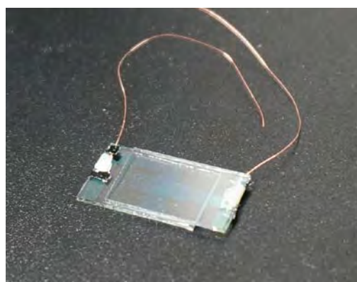
Fast and polarization-independent Phase modulator
